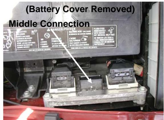
6. Insert the stock connector that you disconnected from the PCM to the EZ module and lock in place with the gray levers.
