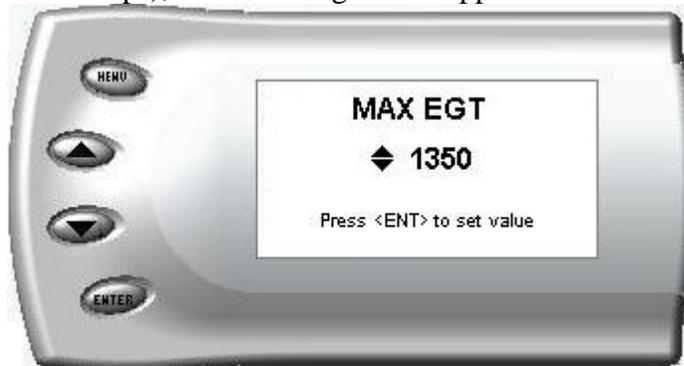
1. Change the Max EGT set point by pressing the up and down arrow keys to select the maximum temperature that you want your exhaust gas temperature to reach, then pressing [Enter]. When the exhaust gas temperature reaches this value, the power delivery will be retarded so as not to allow the temperature to exceed this set value.
