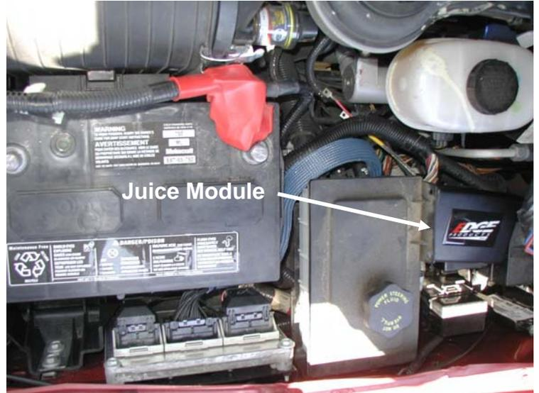
8. Place the Juice module on the right side of the power steering fluid reservoir.
