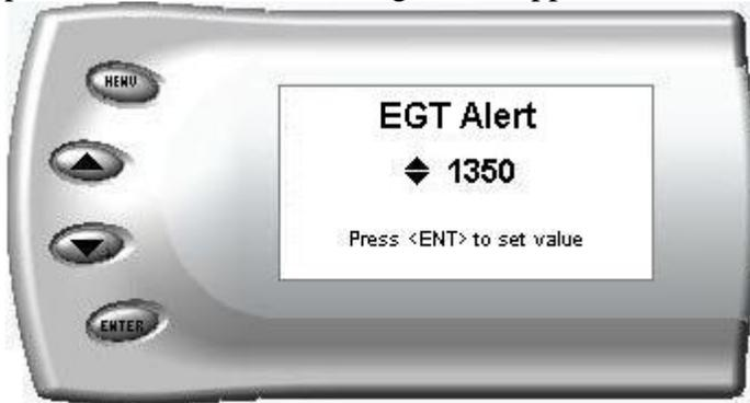
4. Press the up and down arrow keys until you see the desired EGT level at which you want to be alerted and press [Enter] to set that value.
