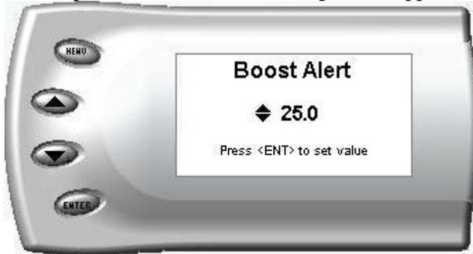
6. Press the up and down arrow keys until you see the desired Boost level at which you want to be alerted and press [Enter] to set that value.
