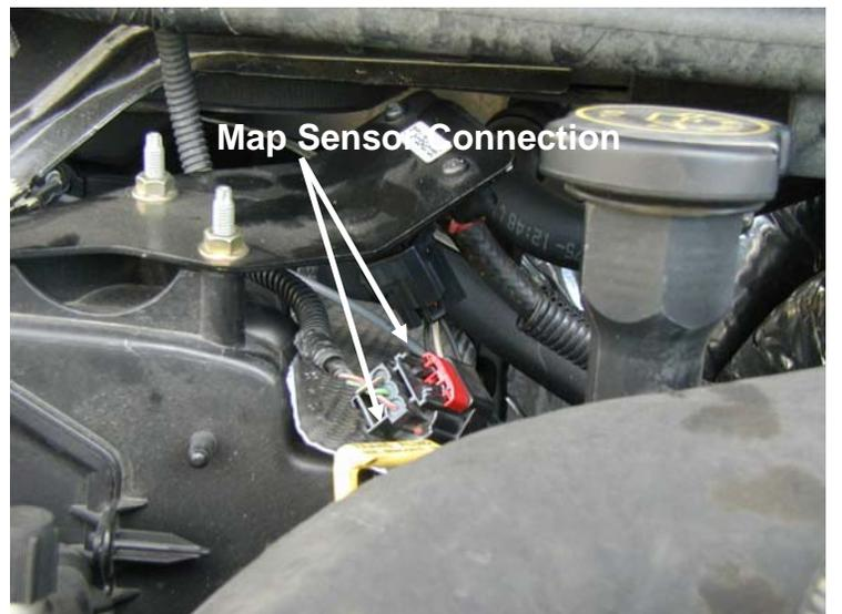
**Notice: Use caution when inserting connector bodies. If connector does not slide smoothly inspect pins and retry.**
